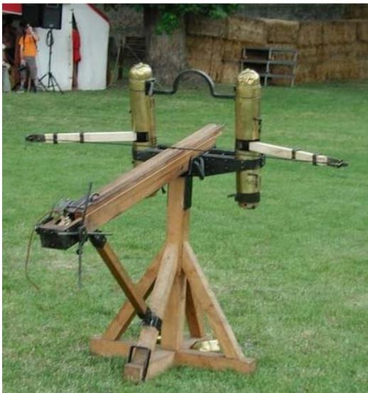
Scorpio—A torsion powered form of crossbow, firing a metal bolt at great force.
