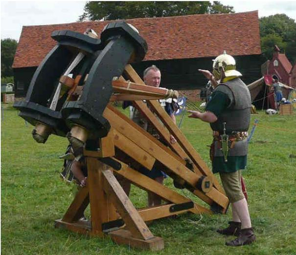
Ballista—A stone throwing machine more like a crossbow than a catapult.
